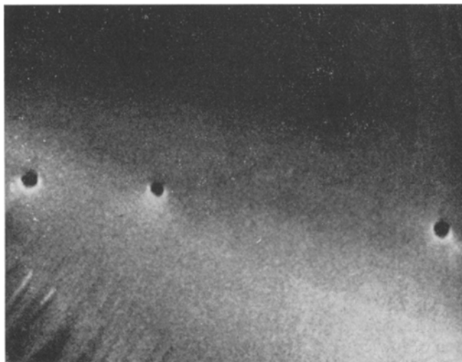
Figure 2 A portion of the fracture surface of a Saphikon filament showing the intersection with three voids ( \times 4000 ).
